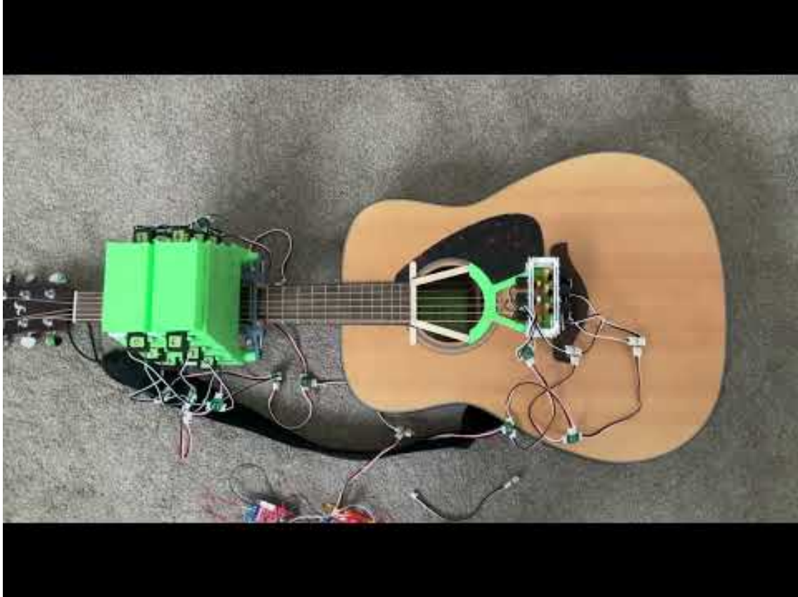
Figure 10: MegCell Difficulty Fretting Close Together https://www.youtube.com/watch?v=JQZKGL_aIY8
